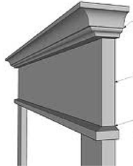
This illustration of a door jamb shows the kind of refined moulded wood products that would come out of a planing mill.
