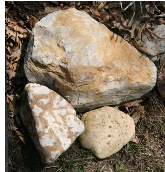
Grand Marais limestone samples, showing the typical range of colours – from whites to soft tans to orangy mottles.
