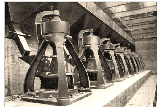
These Griffin-style roller mills, as seen in 1908, were used to grind the clinker into the necessary fine powder. Roller mills rely for their grinding effect almost entirely on the crushing effect of the weight of the wheels, seen at the base of the structures; also note the chutes and hoppers that conveyed the clinker to these machines. (Dylan Moore)
