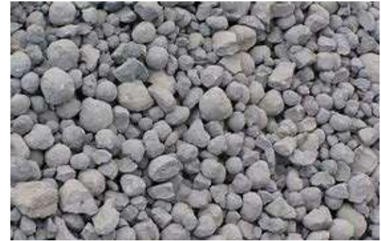
The penultimate result of the cement-making process is called “clinker,” shown here at the point of removal from a kiln. Clinkers are about the size of a marble, and in a final step in contemporary operations are finely ground in a finish mill with a small amount of gypsum, which controls the setting time in the final product. The final cement is an extremely fine powder: one pound of cement contains 150 billion grains.
