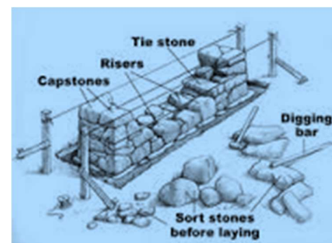
A cut-away diagram showing a stone wall or fence under construction.
