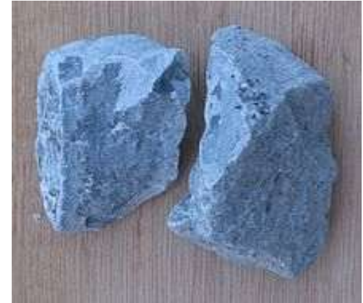
Chunks of calcium carbide, the constituents used in the production of acetylene gas.
